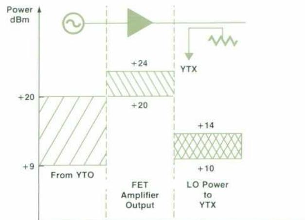
Fig. 4. Variations in the local oscillator power supplied to the mixer diode are compressed by operating the FET amplifier in a saturated mode.
