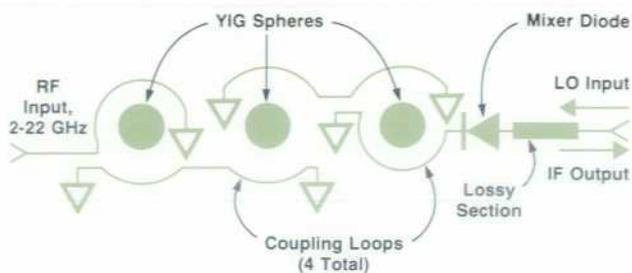
**Fig. 2.** Schematic representation of the YIG-tuned filter and mixer (YTX) used in the 8566A. Although this shows all the coupling loops in the same plane, the two loops for each YIG sphere cross at an angle so coupling occurs only at the resonant frequency of the YIG sphere, which is a function of the dc magnetic field strength.
