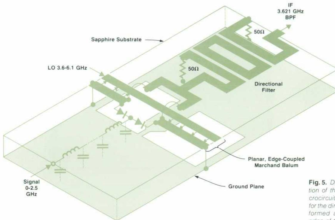
**Fig. 5.** Diagrammatic representation of the second converter microcircuit. The 50Ω terminations for the directional filter are actually formed as thin films along the edge of the substrate.
