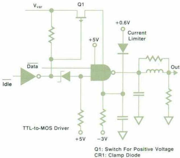
**Fig. 4.** Output drive level is determined by the voltage  $V_{var}$  supplied to the MOS bias input of U1, a TTL-to-MOS driver. Q1 turns off  $V_{var}$  to place the output in the idle (high-impedance) mode.
