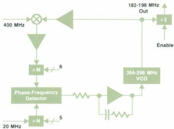
Fig. 3. Block diagram of MIN loop.
