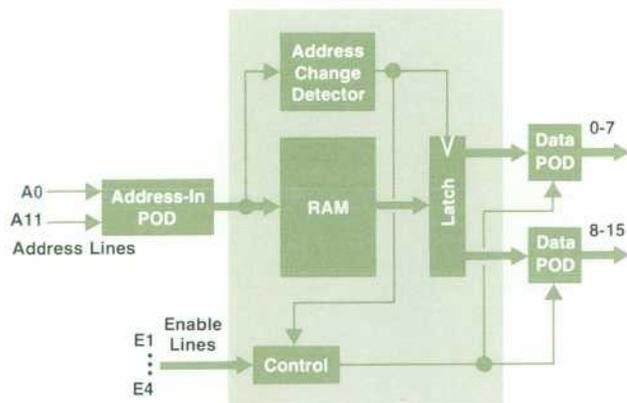
**Fig. 6.** Block diagram of the Model 8170A Logic Pattern Generator operating in the external address mode. Data is output whenever the address-change detector, consisting of exclusive-NOR gates, detects that there has been a change of address. Alternatively, one of the enable inputs may be used as a clock input for timing the data output. A data-valid signal is also generated.
