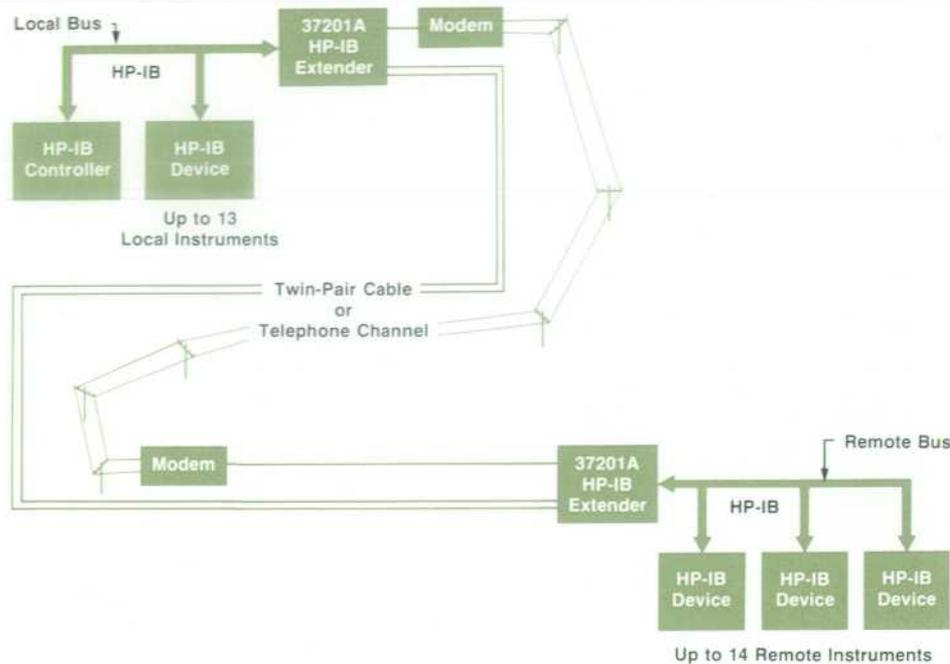
**Fig. 2.** Two distant clusters of instruments are connected through a pair of 37201A HP-IB Extenders in this basic configuration. The controller can communicate with the remote instruments as though they were connected to the local bus.
