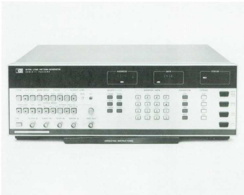
**Fig. 1.** Model 8170A Logic Pattern Generator produces long sequences of 8- or 16-bit parallel digital words as bus stimuli for functional tests of multichannel digital hardware. It operates at clock rates up to 2 MHz, internally or externally supplied.
