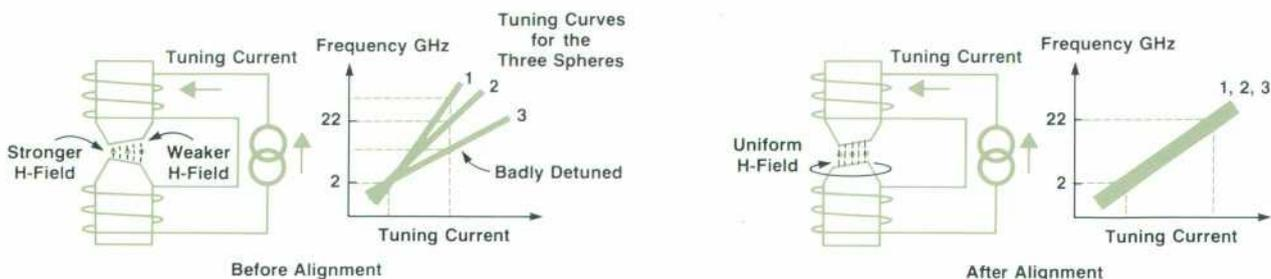
**Fig. 3.** Misalignment of the tuning magnet pole faces, shown exaggerated here, causes the three YIG spheres to have different tuning characteristics. Rotating the pole pieces to bring the tilted faces into parallel alignment achieves identical tuning characteristics for the three spheres.
