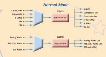
The normal mode is designed to convert from one video format to another and from one audio format to another. Both the audio and the video signals are synchronized to the input genlock reference signal. Video and audio adjustments can be carried out on the input signals.
