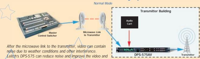
audio quality. The DPS-575 also provides a trouble slide and a voice over in the transmitter building. During a loss of video the DPS-575 can automatically switch to an alternate source or trouble slide.
